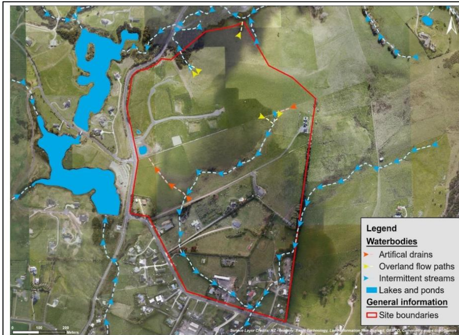
Figure 13: Showing the general hydrological patterns as observed on site during site field visits
